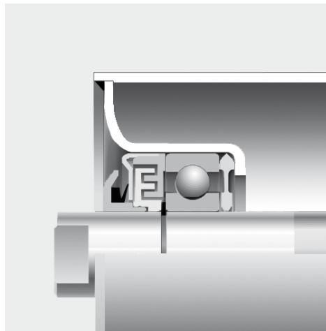
Section through sealing
