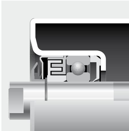
Section through sealing
