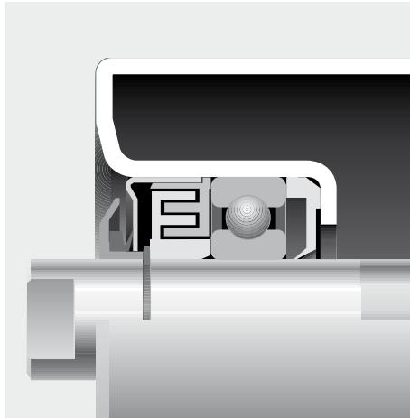
Section through sealing
