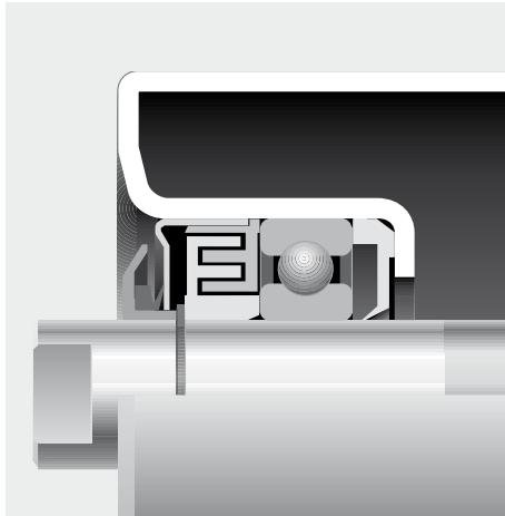
Section through sealing
